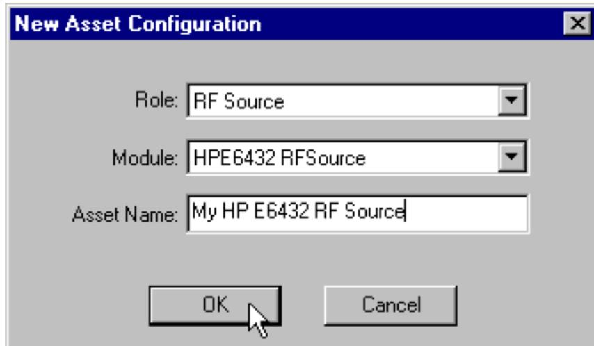
5. The left-hand window pane should now show the newly added asset as an RF Source that can be selected and used by the current configuration.
