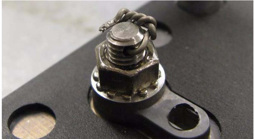
To remove a Safety Wire, untwist the wire and pull it through the hole in the Shoulder Screw.
