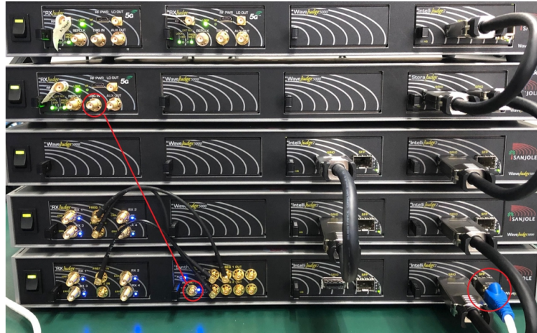
NSA WaveJudge 5000 Chassis Front Panel Connections
