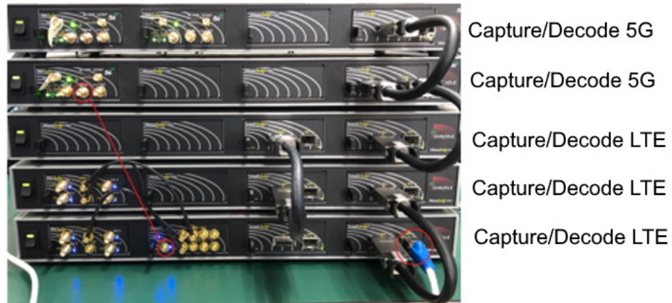
Example 5: NSA (4G LTE and 5G) Front Panel Configuration
