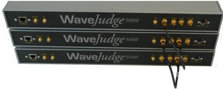
Three WaveJudge 5000 Chassis Connected via Sync In and Sync Out
