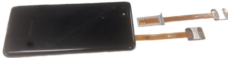
CipherJudge - SIM Tray Adaptor Plugged Into Cell Phone
