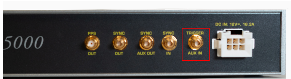
WaveJudge Back Panel: Trigger - AUX IN Connection
