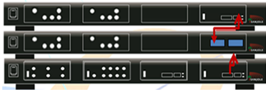
Example 4: Combined LTE and 5G System Using Three Chassis, Four 40 MHz Ports, and Four 800 MHz Ports
