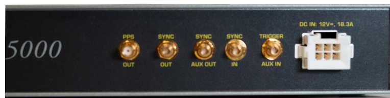
Back of WaveJudge 5000 - Right Side Clock Connections
