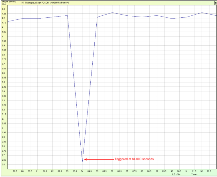
IntelliJudge Throughput Chart Showing Trigger
