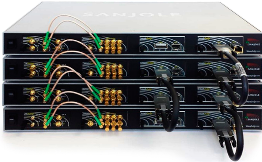
Four WaveJudge 5000 Chassis Interconnected via SRIO
