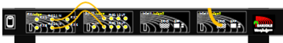
Example 1: 4G LTE Chassis with Four 40Mhz Ports Connect to RxJudge 5G
