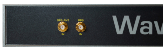
Back of WaveJudge 5000 - Left Side Clock Connections
